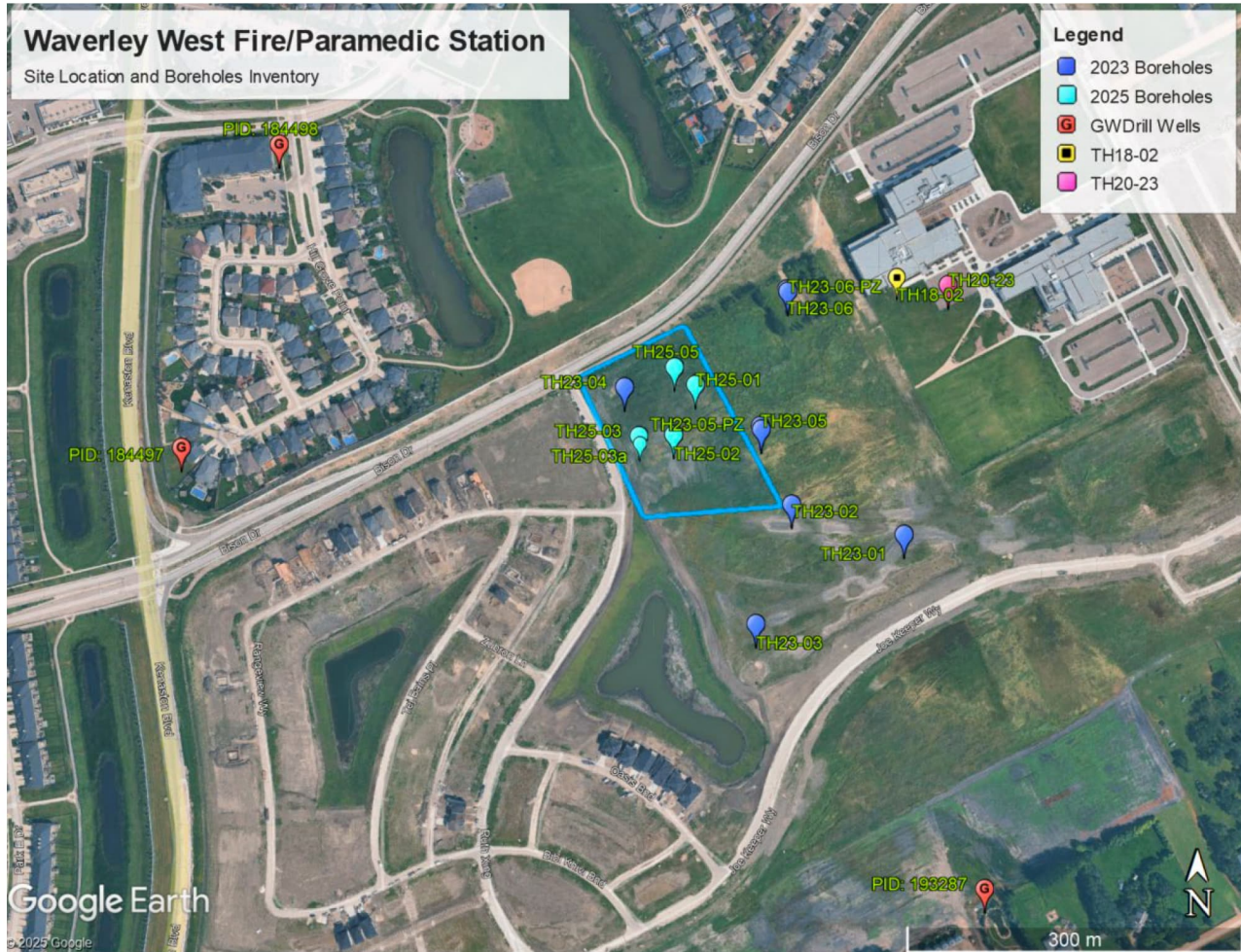
FIGURE 1: PROJECT AREA AND LOCATION OF BOREHOLES REVIEWED
